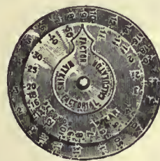
FIG. 72.—Watkins's Factorial Calculator.
